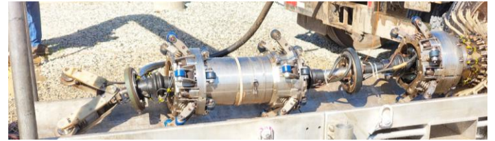
Pipeline Inspection Gauge (PIG) used for Integrity Assessments
