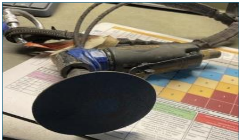
Figure 3: Non-intrinsically safe tools used in explosive atmosphere.
