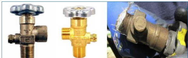
Figure 2: Under-rated valves used with high-pressure gas cylinders.
