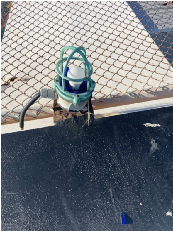
Figure 2. Photo (left) of the damaged center perimeter light shortly after the accident (Source: Walter Oil and Gas). Photo (right) of the same light assembly after it was removed from the helideck (Source: NTSB).
