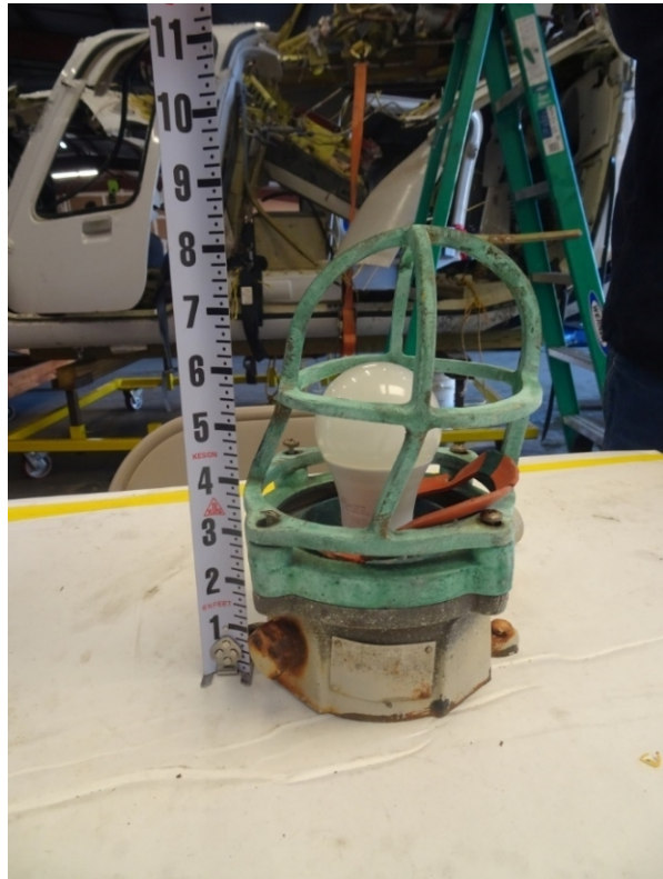
Figure 2. Photo (left) of the damaged center perimeter light shortly after the accident (Source: Walter Oil and Gas). Photo (right) of the same light assembly after it was removed from the helideck (Source: NTSB).
