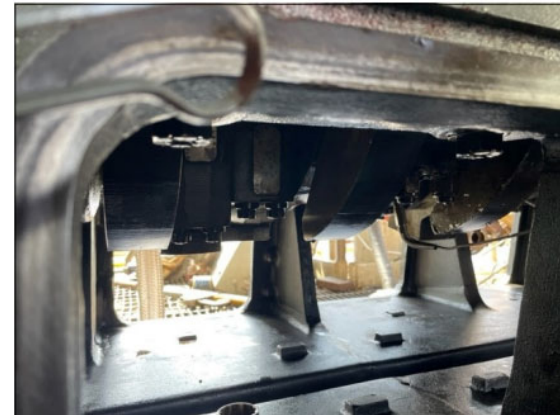
Description: Side view of compressor block with rod caps.
