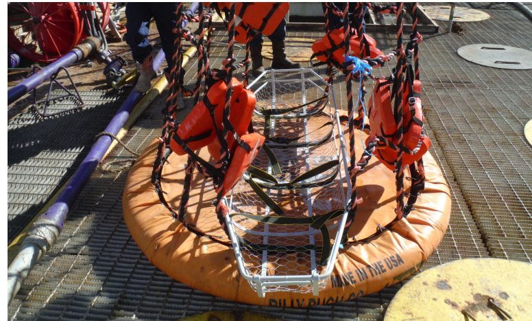
Stokes litter that had no available rigging to be lifted other than riding on a personnel basket
