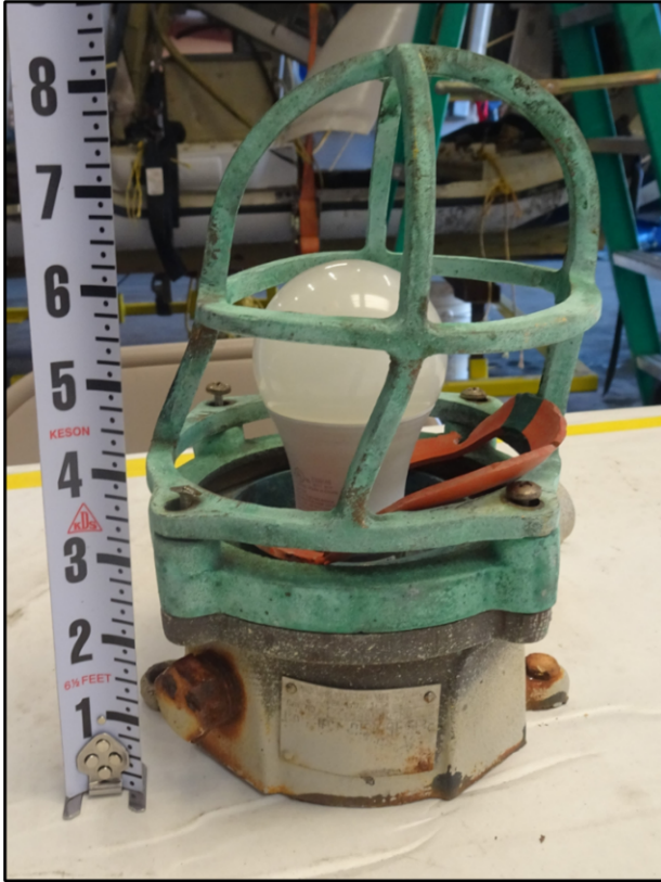
Image 3a (left) – Damaged perimeter light from west edge of helipad
