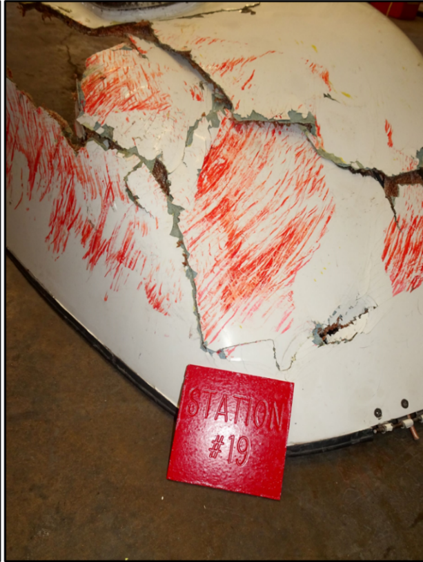
Image 3a (left) – Damaged perimeter light from west edge of helipad
