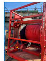
Incident 1: The spot where the contractor's right thumb was pinched between the ball valve and the hose head.
