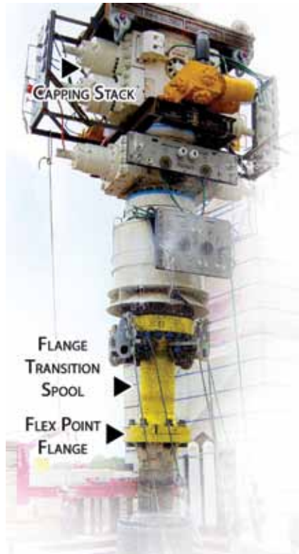
The Capping Stack, connected to the well via the transition spool to the Lower Marine Riser Package and blowout preventer. Successful installation of the Capping Stack represented the completion of the closed system that allowed for initial shut-in of the well flow.
