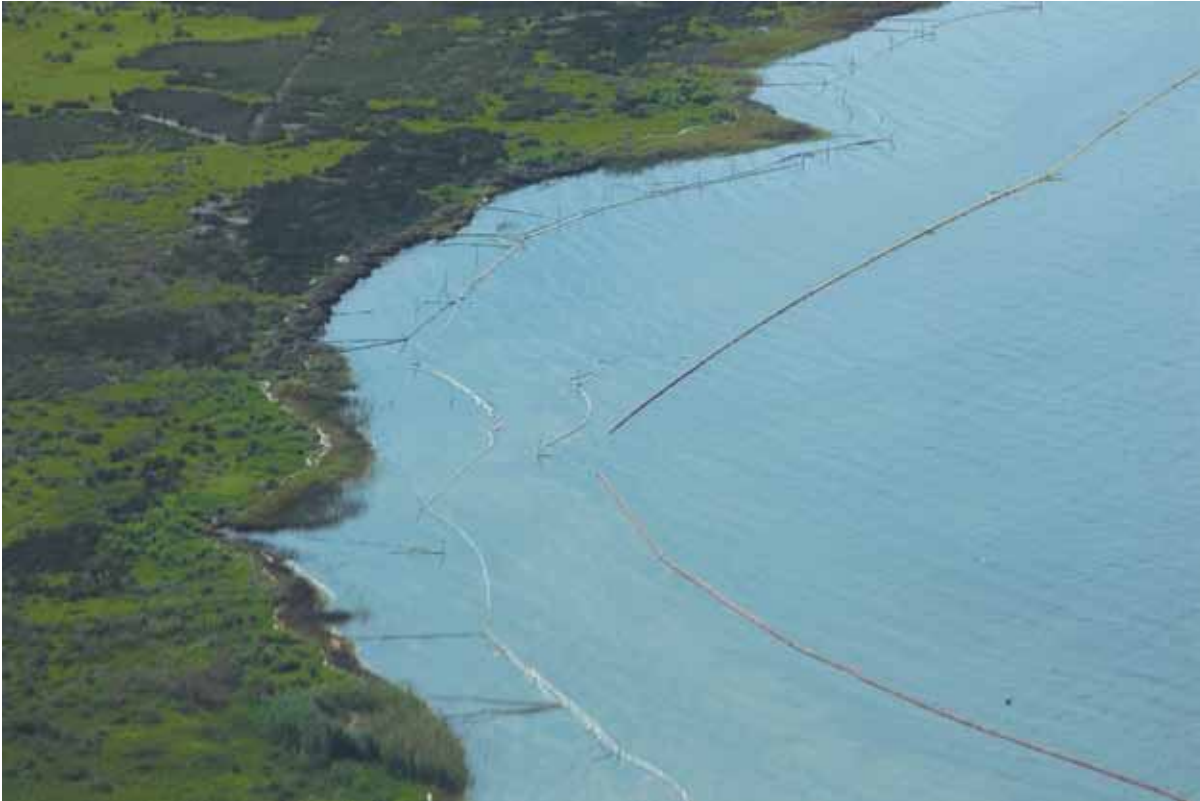
Layers of boom protect a marsh. Teams of 16 to 20 responders made up the more than 2,500 person marsh cleaning operation, which used proven techniques for effective and non-invasive remediation.
