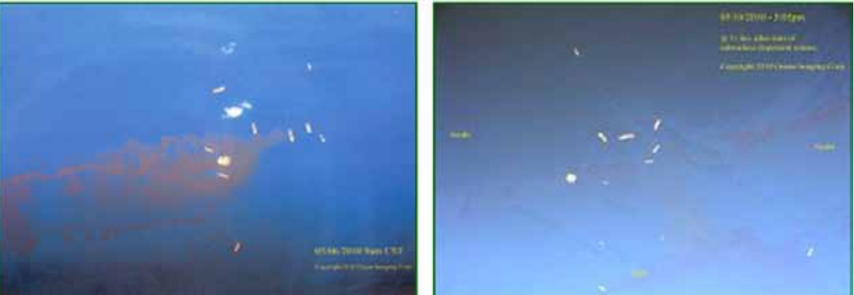
surface oil above the source before and after subsea dispersant injection. Testing found that dispersant use reduced the level of oil and volatile organic compounds (VOCs) at the surface, enhancing safety and making subsea containment efforts possible.
