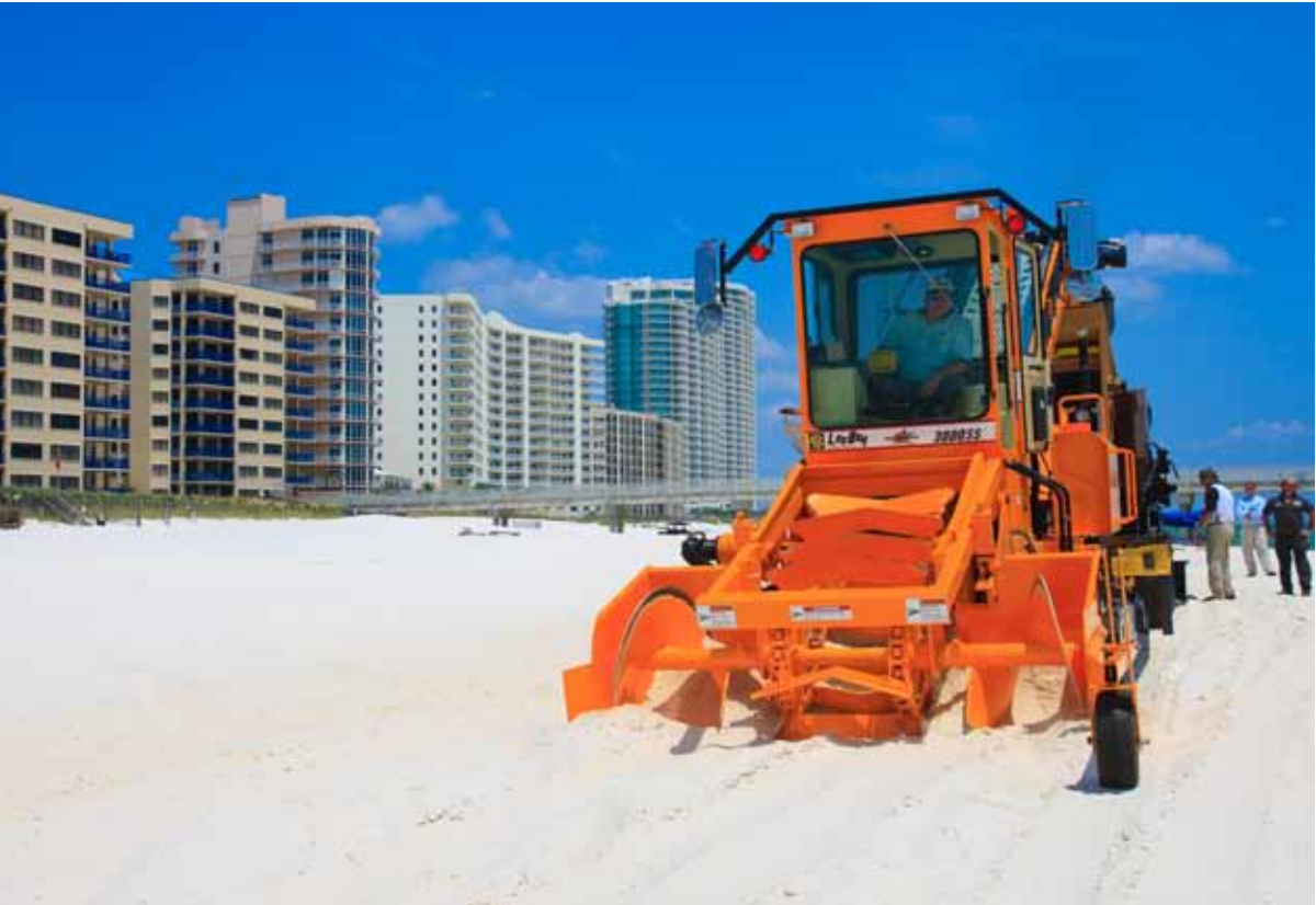
A Sand Shark developed specifically for the beach clean-up effort, using continuous improvement methodology, allowed deeper digging to capture oil below the surface.
