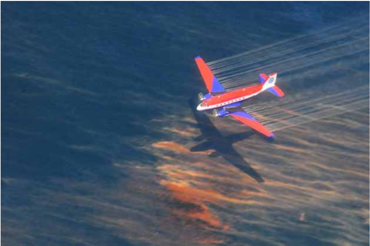
A plane targets dispersant to break up oil before it reaches shore. The response team increased the effectiveness of dispersant application through process and supply chain improvements, the use of imaging and other technologies, and the establishment of sampling and monitoring programs.
