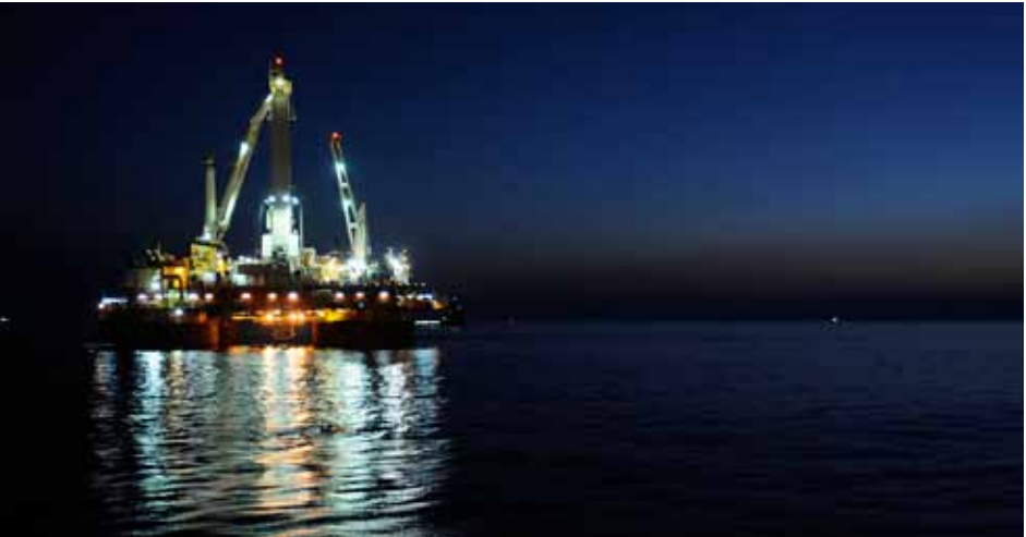
The Q4000, a multipurpose vessel used both for a range of subsea containment activities and for collection and disposal of oil.
