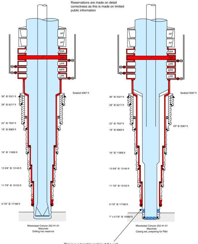
This is a vulnerable section of the well. If the cement above the cap rock is not good there will be a channel travelling all the way to the well head exposing the 16" casing and the 9 7/8" hanger seal assembly.
