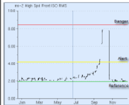
(a) Inner ring fault detected in gearbox intermediate shaft bearing
